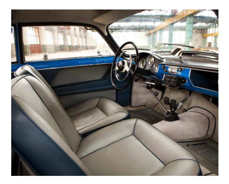
There was no glove department cover, no sun visors, and no rear seat. The Veloce seats were thinner, albeit foam-padded, and mounted on a delicate tubular frame. A central gearshift was employed instead of the columnmounted gearshift.
